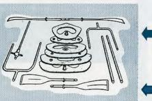
The shaped plywood frames for both kayaks are fitted together by lengths of metal pipe which also serve to stabilize the craft. The entire framework fits into a one-man haversack.
