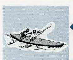
THE TWO-MAN KAYAK is a collapsible, portable boat made of a plywood frame covered by rubberized canvas. Assembled, the boat weighs 104 lbs., is 16½ ft. long, has a beam of 34 in. and a depth of 13 in. It can be assembled by two men in less than five minutes.
