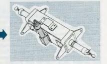
THE BEACH SAND AUGUR takes a cubic sample of sand 8 in. long and % in. in diameter. The sand is transferred to plastic tubes carried in a bandolier.
