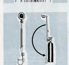
THE UNDERWATER COMPASS is a standard waterproof compass fitted into a holder which is attached to the Lambertson Unit. A joint enables the swimmer to raise the compass to eye level or push it down flush to his body. It does not interfere with swimming in either position.
