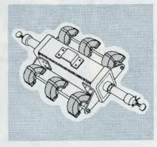
The Limpet is most effective when used about 5 ft. below the water surface, its charge being sufficient to blow a hole about 25 sq. ft. in a merchant vessel. The Limpet may be attached under water either by a swimmer or from a small boat with the aid of an extendable placing rod. A range of time delays permits the operator to make his escape.
