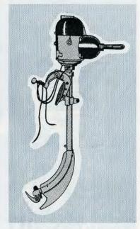
THE ELECTRIC MOTOR is driven by a 12-volt, 120-ampere battery. Silent in operation, it is used as motive power for the surfboard.
