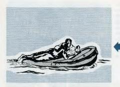
THE TWO-MAN SURFBOARD is a pneumatic rubber surfboard, 10½ ft. long, 3 ft. 7 in. wide, weighing about 310 lbs. A compressed air cylinder inflates it in a few minutes. A battery-driven 34 horsepower motor with a speed of 5 knots and a range of 10 miles can be attached. The surfboard carries two men and their equipment, the equivalent of 900 lbs.
