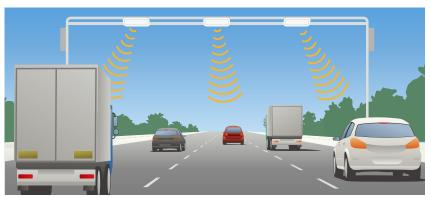
Electronic Toll collection uses networked readers that scan for RFID enabled transponders. Some readers work at highway speeds.
