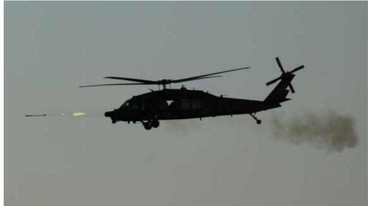
The **MH-60K** is a highly modified twin-engine utility helicopter based on the basic UH-60 Black Hawk airframe but developed specifically for the special operations mission. Improvements include an aerial refueling capability, an advanced suite of aircraft survivability equipment and improved navigation systems, including multi-mode radar to further improve pinpoint navigation in all environments and under the harshest conditions.
